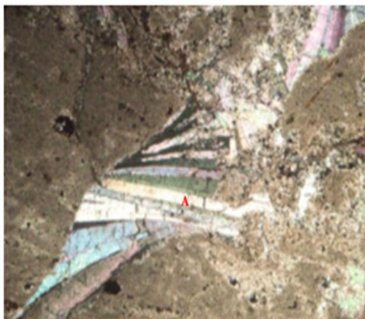
Plate.5. Photomicrograph shows laths of anhydrites have completely filling porosity(A). Intertidal / Supratidal Anhydrite /Dolomite facies: Bioturbated Dolomite Mudstone Microfacies
